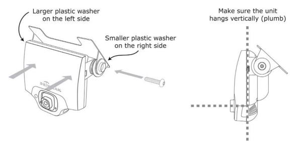
The **Large Plastic Washer** on the left side of the bracket is designed to partially cover the RJ45 Interconnect cable so that it cannot be unplugged by the driver. The plastic washers can be easily removed from the metal bracket after removing the screws. Make sure the larger of the two washers is on the left (power connection) side of the bracket.
